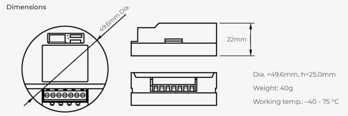
Note: The module requires a 12 VDC power supply with a nominal power of at least 3W
